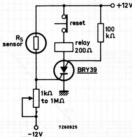
$R_S$  must be chosen in accordance with the light, temperature, or radiation intensity to be sensed; its resistance should be of the same order as that of the potentiometer.
