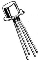
Silicon N-channel junction field-effect transistor
