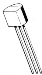
NPN silicon annular, plastic encapsulated transistors for low-cost amplifier and oscillator applications at VHF and UHF.
