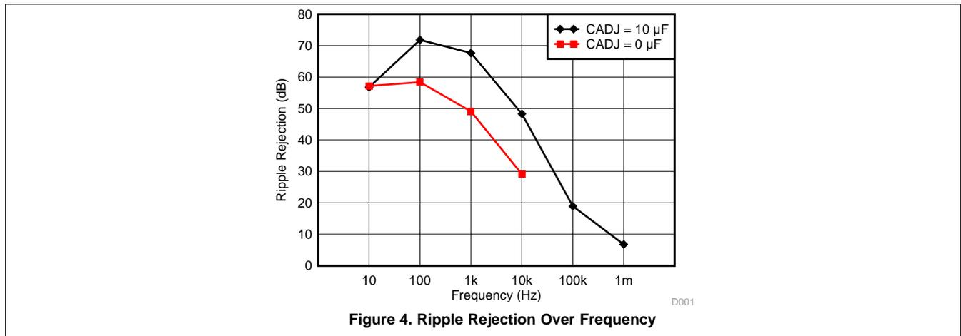
Figure 4. Ripple Rejection Over Frequency
