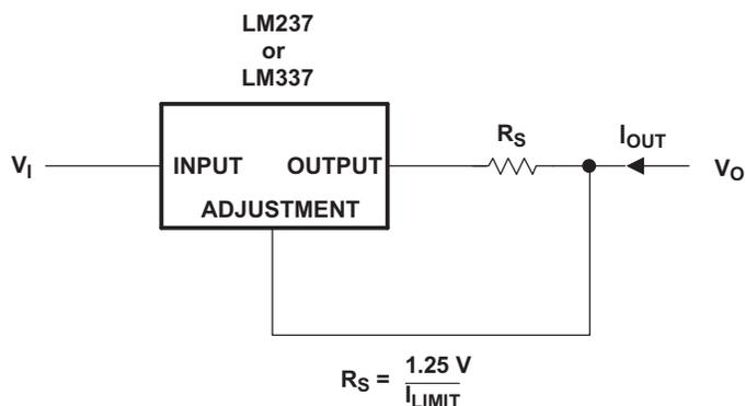
Figure 2. Current-Limiting Circuit
