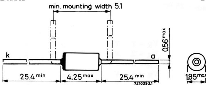
Cathode indicated by coloured mark or by broad band if colour coded (see General Section)
