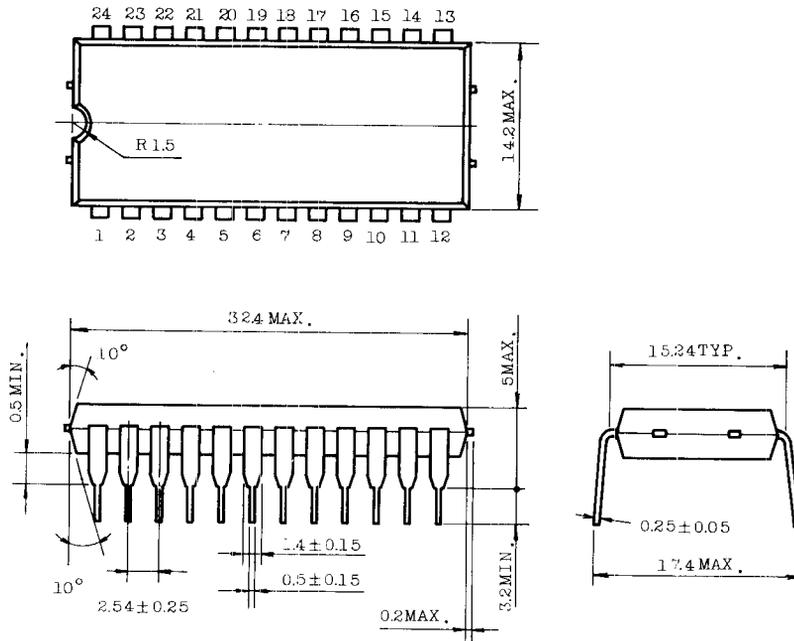
Note : Each lead pitch is 2.54mm. All leads are located within 0.25mm of their true longitudinal position with respect to No.1 and No.24 leads.
