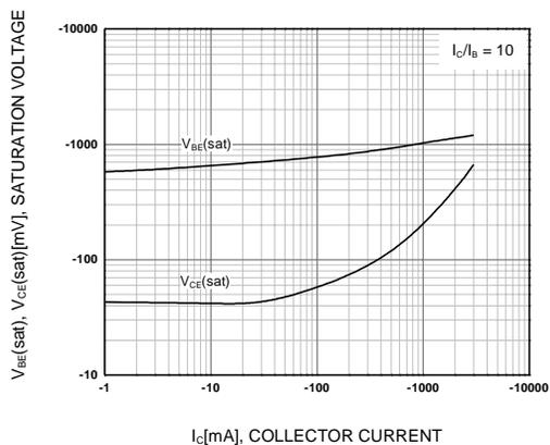
Figure 2. Base-Emitter Saturation Voltage
