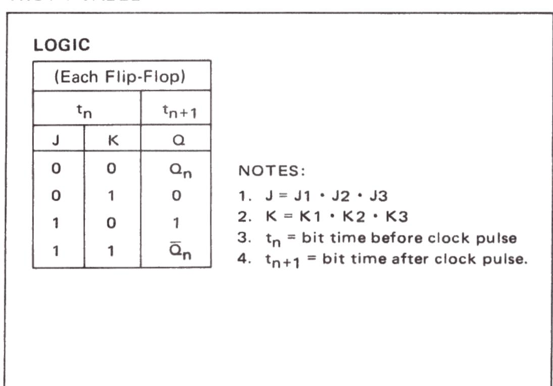
Low input to preset sets Q to logical 1 Low input to clear sets Q to logical 0 Preset and clear are independent of clock
