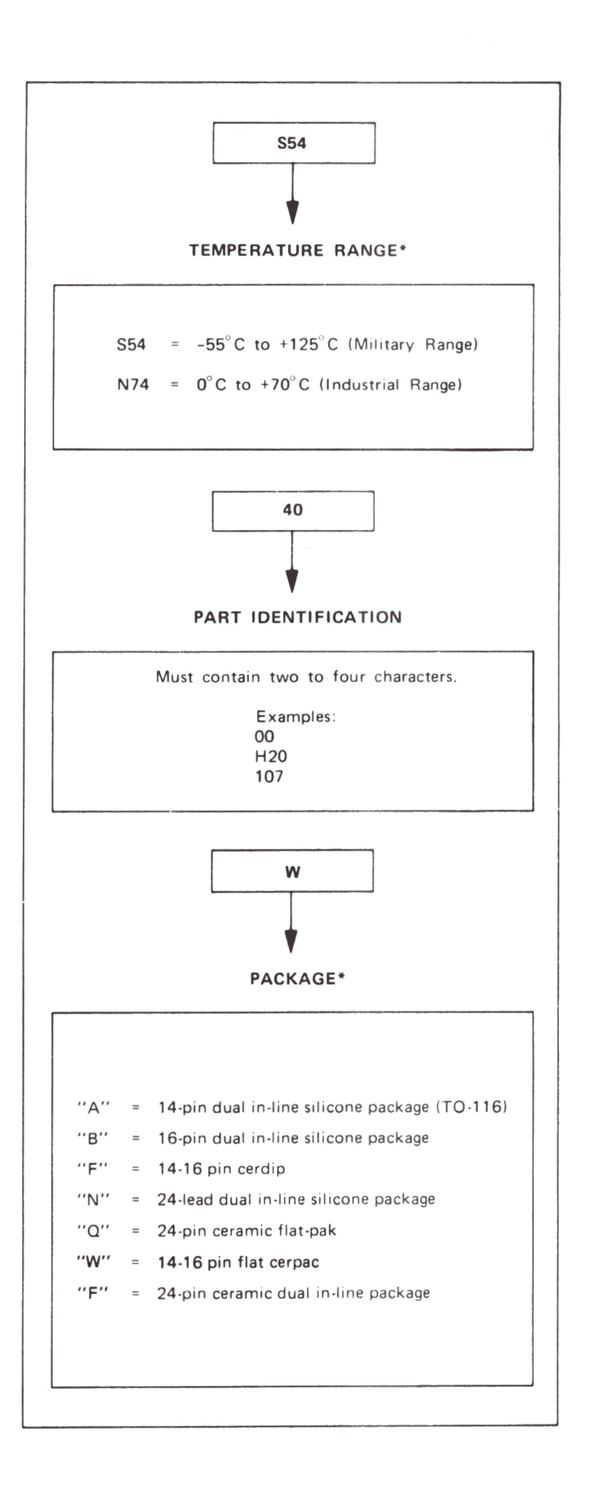
\*Availability of a circuit device in a particular package and temperature range is indicated on the appropriate device. Electrical Characteristics Data Sheet is shown in Section 2 of this handbook.
